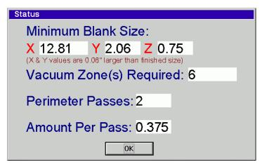
Selecting the Status button will display the dialog box seen at the left. This shows the minimum blank size needed, number of vacuum zone needed to be open, and the number of passes and the amount of material per pass that will be machined for the information entered in the main field.
